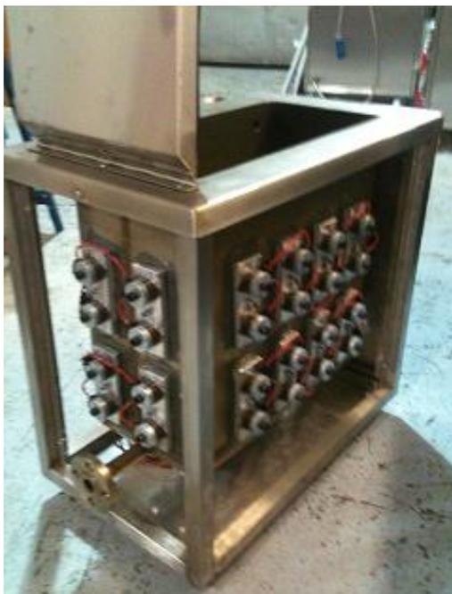
*Acoustic Cavitation Reactor (ACR) with sides removed to show the ultrasound generators*
